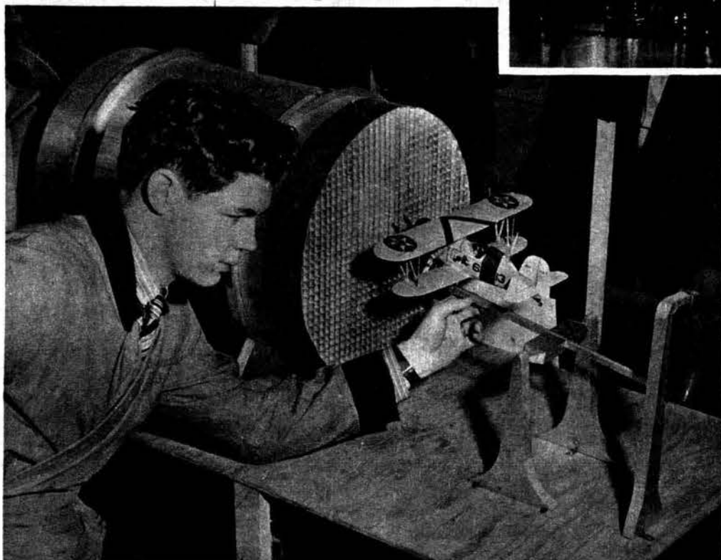
Here Richard Walton, a winner of the Science Fair conducted at the Pennsylvania Science Center, works with his homemade wind tunnel. The lift of the airplane is registered by the spring scale at the extreme right.
