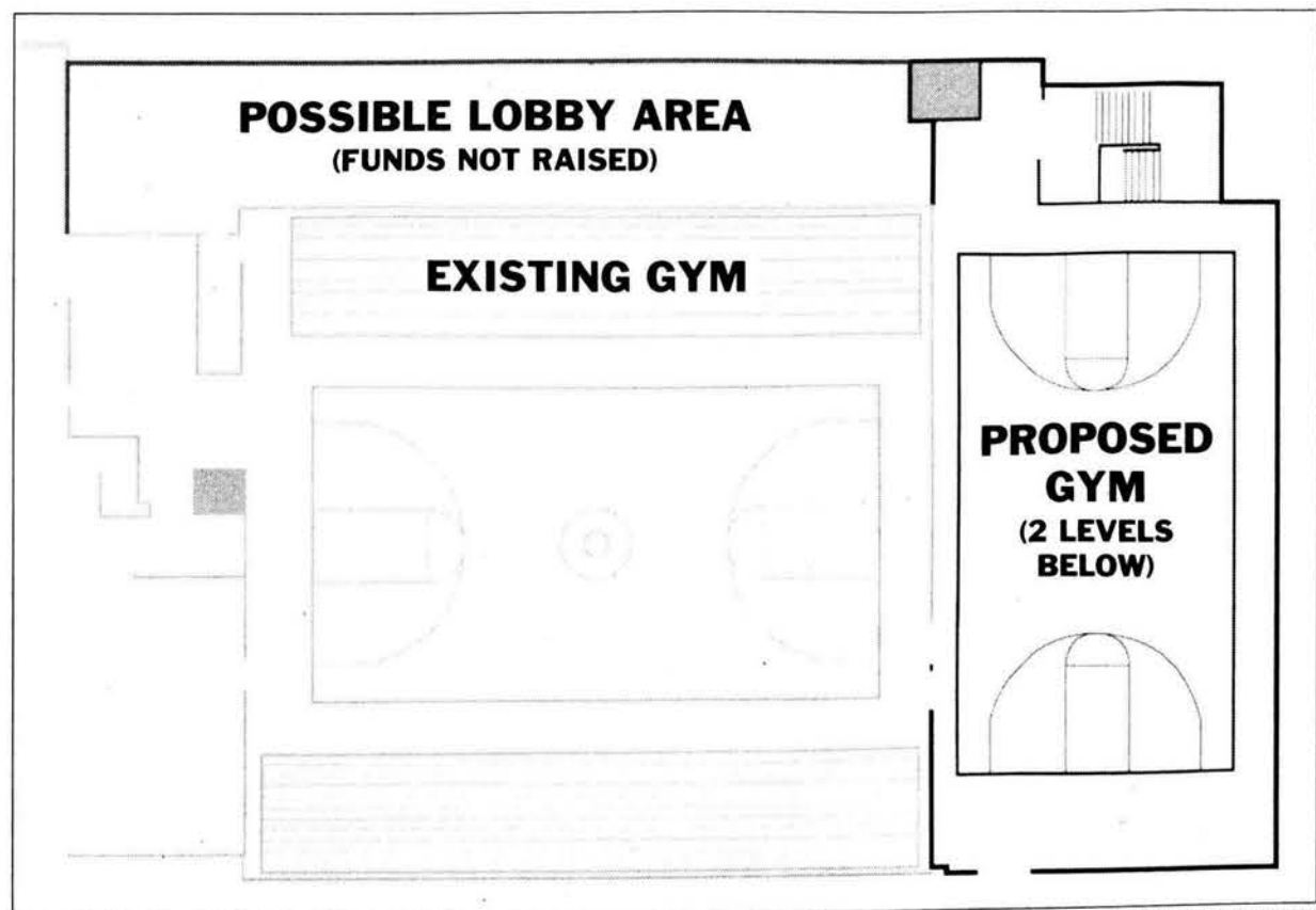
Plans courtesy of DLR GROUP The top floor of the proposed gym addition. The top floor may even have wooden floors installed. The middle floor, directly beneath the gym, is currently cast as a weight room, and the bottom level will probably be used for wrestling and aerobics.
