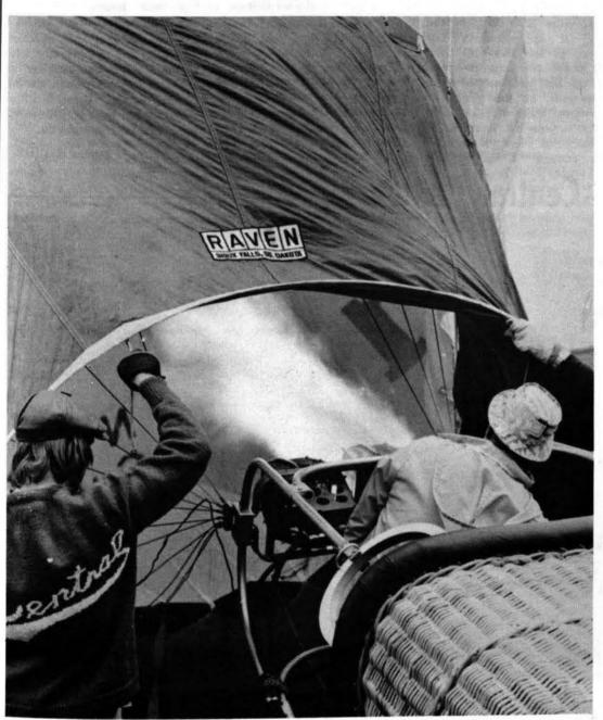
After using a gas-motor fan to inflate the balloon, the propane burners are lit to warm the air inside, causing the balloon to rise, and then it's up, up, and away . . .
