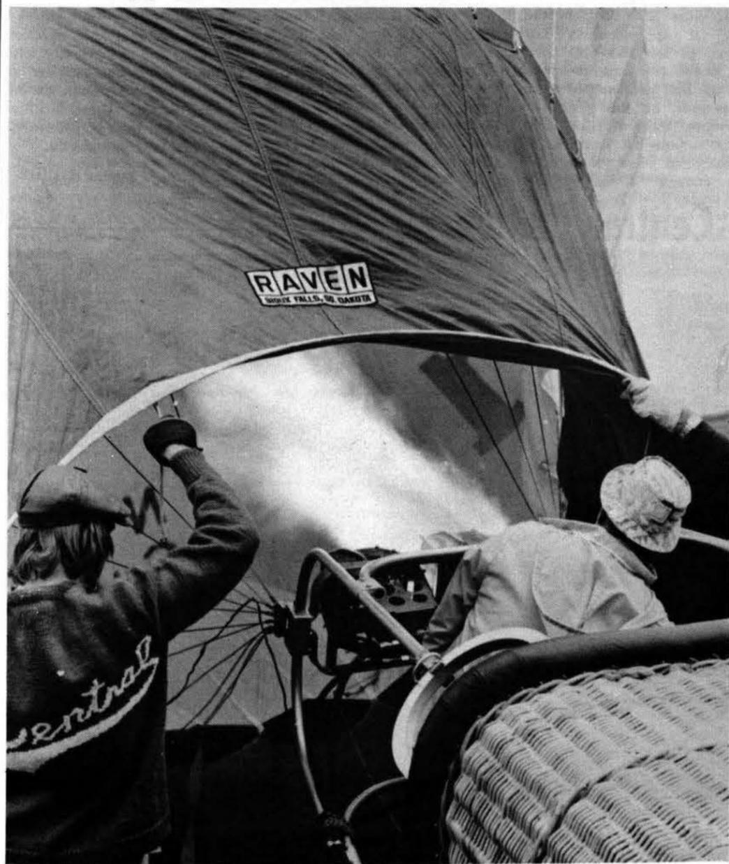
After using a gas-motor fan to inflate the balloon, the propane burners are lit to warm the air inside, causing the balloon to rise, and then it's up, up, and away . . .
